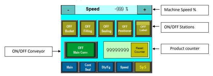
The speed of the machine can also be adjusted on this screen. Use the top window to increase or decrease the speed to suit the other equipment connected to the machine.
